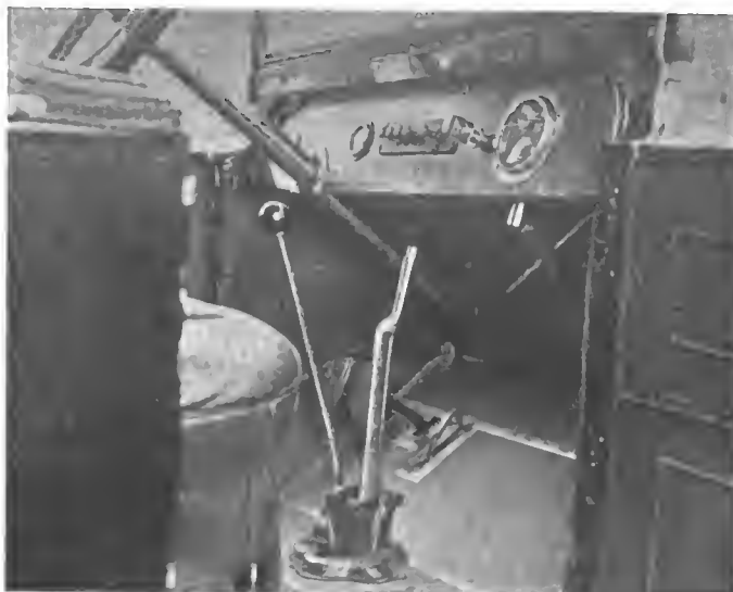
Cowl board and control features in the new Buicks as found on the large four and six. Note mounting of speedometer in cowl board face
